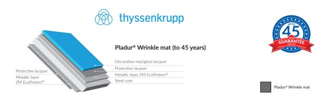
**Pladur® Wrinkle mat** - thick-grain, double-layer coating system, with colours according to well-known patterns and min. coat thickness 35 microns. The sheets meet the requirements of class A2 in accordance with the Commission Decision 96/603/EC on fire protection and may be used in the corrosion category C4 according to the standard EN ISO 12944-2.
